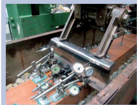
Fig. 6: Scissors-lever vibration test at Munich University of Technology (Photo: Munich University of Technology)
