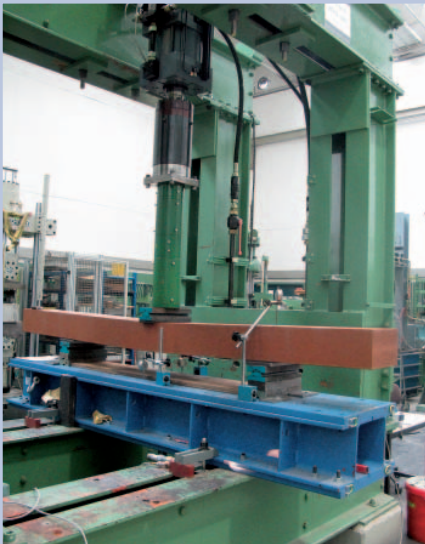
Fig. 8: Static test in the middle of a sleeper (Photo: koocoo consulting)
